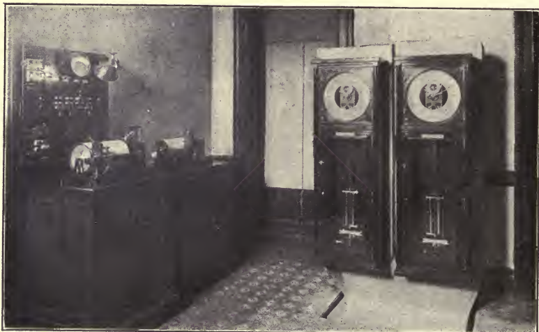
TRANSMITTING CLOCKS, CHRONOGRAPHS AND SWITCHBOARDS USED IN THE U. S. NAVAL OBSERVATORY IN SENDING OUT THE TIME TO THE COUNTRY
